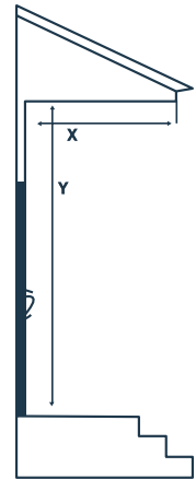
Figure 1: where X is the length of the overhang required and Y is the distance from the bottom of the door to the base of the overhang.
