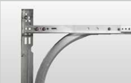
15" Radius Track 14¾" Min. Headroom Req.
