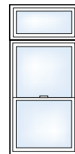
A Single Hung mullered with a Picture window above. A Geometric window may be substituted for the Picture window.
