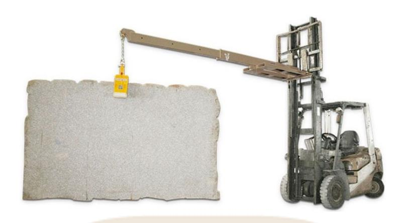
Be sure to use the proper personal protective equipment when lifting and handling slabs. A forklift with a slab boom or lifter (clamp) should be used when moving individual slabs. When moving multiple slabs at once, a crane should be used if possible. Prior to moving slabs, it is important to have an idea of the weight of the bundle to ensure that you do no exceed to equipment's rated capacity.
