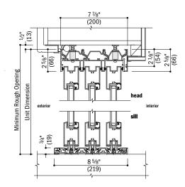
**Vertical Section** On-Floor Drainage Sill
