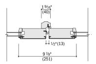
**Horizontal Section** Astragal, Lead Panel-Lead Panel
