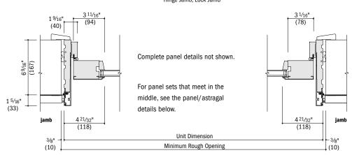
**Horizontal Section** Hinge Jamb, Hinge Jamb
