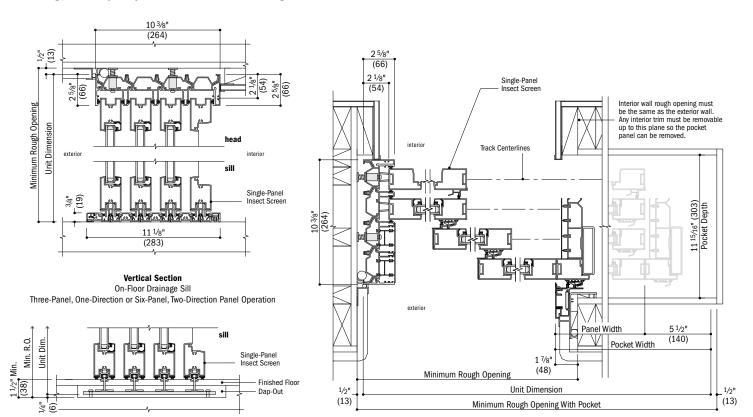
**Vertical Section** Flush Sill Three-Panel, One-Direction or Six-Panel, Two-Direction Panel Operation
