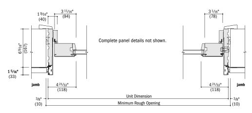
**Horizontal Section** Hinge Jamb, Lock Jamb
