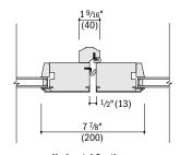
**Horizontal Section** Astragal, Lead Panel-Lead Panel
