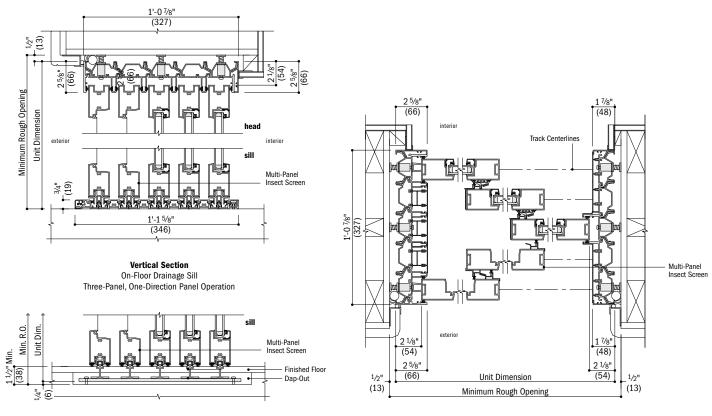
**Vertical Section** Flush Sill Three-Panel, One-Direction Panel Operation
