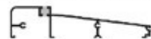
Standard Inswing Sill Thermally broken - 5-5/8" width. Optional extenders for larger wall sizes.
