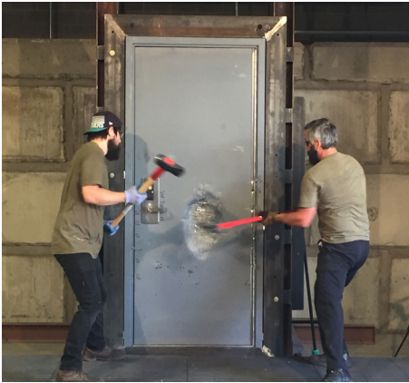
Image from actual forced entry testing
