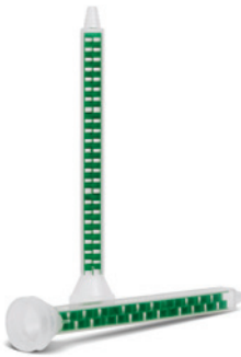
QWIK-MIXERS (24/PK) Required dispenser for Fast Cure and Slow Cure AZEK adhesive products. The resin and catalyst blend together as they travel down the tube to the applicator tip. Ensures 1:1 ratio mix and provides easy adhesive application. 24 per pack. 50 ml: AAD50MLSQM 220 ml: AAD220MLQM
