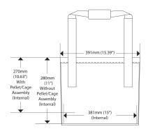
The CookTek® ThermaCube™ thermal delivery bag is constructed of nylon and VaporVent™ material with Velcro closures and a transparent ticket window. Fully equiped with four polycarbonate stiffeners for the sides of the bag, and a divider to split the bag into two chambers, offering a versatile delivery solution. The ThermaCube™ thermal delivery bag has been specifically designed for use on the ThermaCube™ induction charging bases only - not compatible with CookTek PTDS components.
