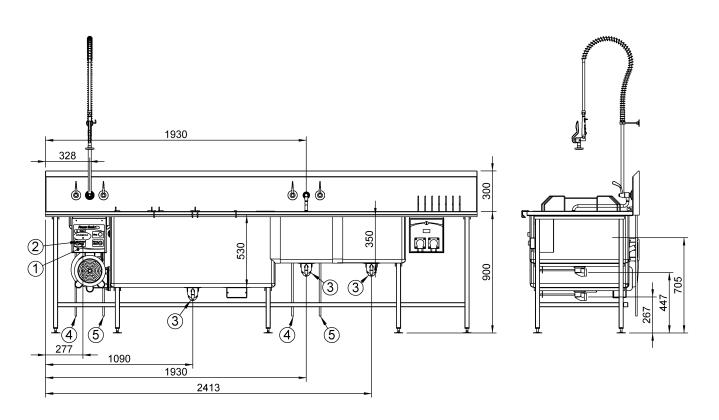
1 Electrical Connection: Single Phase 240v 20amp 50Hz
