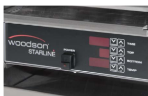
Belt and temperature control
