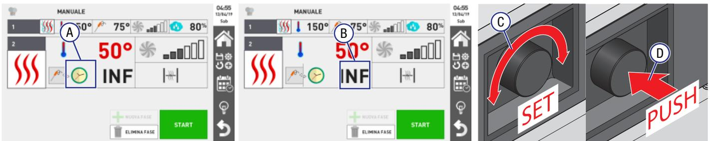
**Note:** To make the oven works continuously, Touch the time field and turn the navigation dial to the left until the display shows INF. If the Delta T function is required, set the temperature of both the core probe and Delta T.
