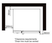
\* Heat Source: 500mm clearance from an external heat source is required in order to protect the oven control components and allow access to the service panel. For clearances under 500mm, it is mandatory for Stoddart hast shields to be fitted while still maintaining a minimum clearance of 300mm to provide access to the service compartment. Failure to adhere to minimum clearances may void the oven warranty or add service costs due to lack of access.
