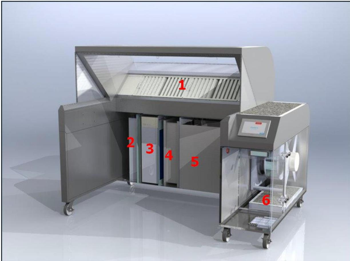
1. Mechanical double stage pre-filtration – KSA cyclonic filters & mesh filters (>95% at 10um)
