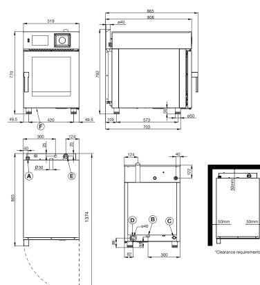
\*Heat Source: 500mm clearance from an external heat source is required in order to protect the oven control components. For clearances under 500mm, it is mandatory for Stoddart heat shields to be fitted while still maintaining a minimum clearance of 50mm to allow access to the unit. Failure to adhere to minimum clearances may void the oven warranty or add service costs due to lack of access.
