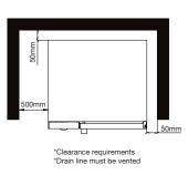
\* Heat Source: 500mm clearance from an external heat source is required in order to protect the oven control components and allow access to the service panel. For clearances under 500mm, it is mandatory for Stoddart heat shields to be fitted while still maintaining a minimum clearance of 300mm to provide access to the service compartment. Failure to adhere to minimum clearances may void the oven warranty or add service costs due to lack of access
