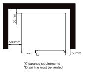
\* Heat Source: 500mm clearance from an external heat source is required in order to protect the oven control components and allow access to the service panel. For clearances under 500mm, it is mandatory for Stoddart heat shields to be fitted while still maintaining a minimum clearance of 300mm to provide access to the service compartment. Failure to adhere to minimum clearances may void the oven warranty or add service costs due to lack of access.
