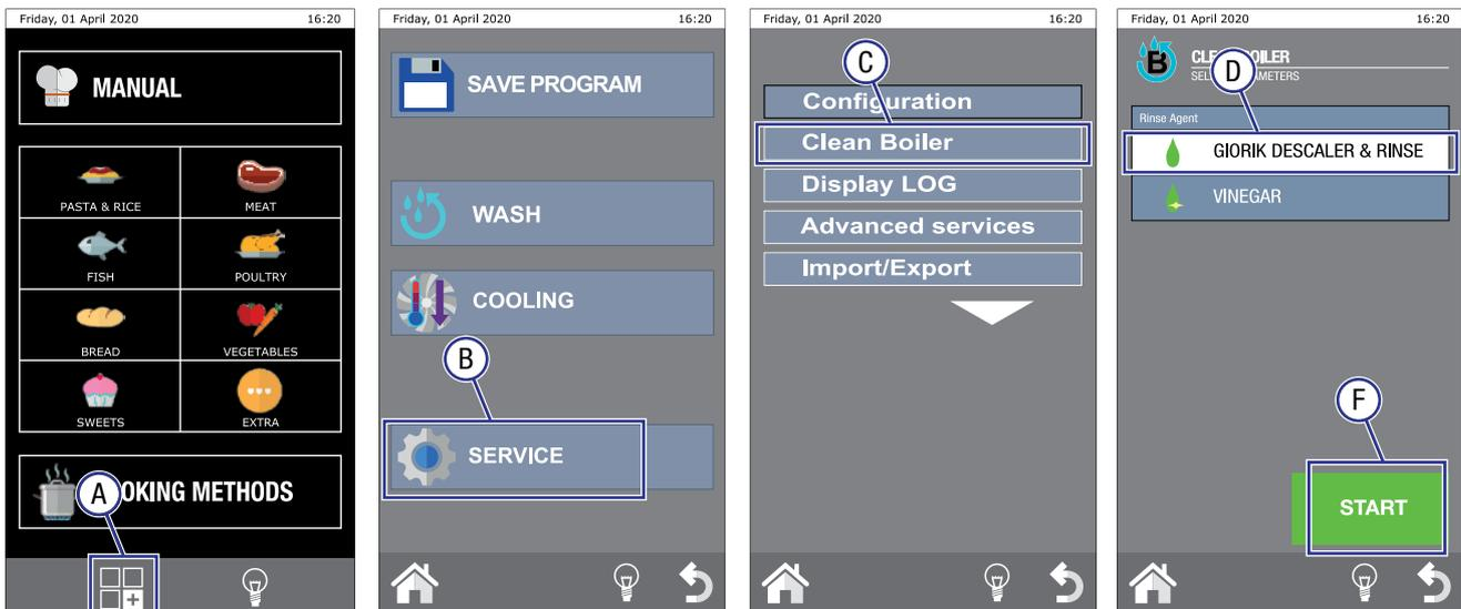
**Note:** A display window indicates the progress of the operation, which occurs in three steps: Getting Ready, Descaling phase and Rinse.
