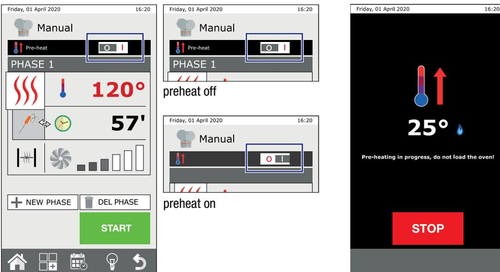
This screen displays the current temperature in the chamber (which will increase gradually) and warns that preheating is in progress. The oven requires the set temperature to be reached before introducing food into it. If necessary, the value can be changed by touching it and turning and pressing the navigation dial to the right.
