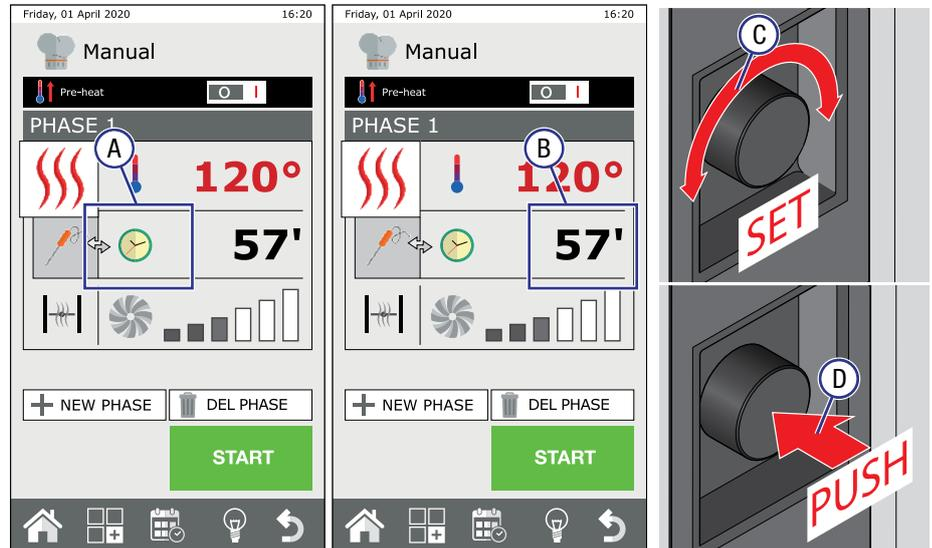
**Note:** For the oven to run continuously, touch the time field and turn the navigation dial to the left until the display shows INF.
