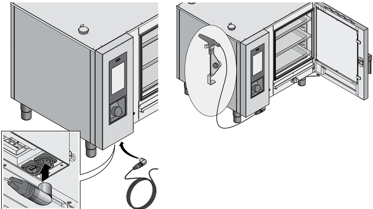
**Note:** When not in use, place the probe back into the magnetic support on the left side of the oven.
