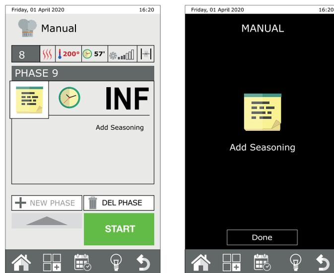
**Note:** While the message is displayed, the oven keeps running with the set temperature until “Done” is pressed (If programmed, the next phase will start).
