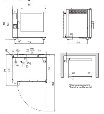
Heat Source: 500nm clearance from an external heat source is required in order to protect the oven control components and allow access to the service panel. For clearances under 500mm, it is mandatory for Stoddart heat shields to be fitted while still maintaining a minimum clearance of 300mm to provide access to the service compartment. Failure to adhere to minimum clearances may void the oven warranty or add service costs due to lack of access.
