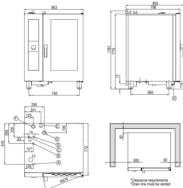
**Heat Source:** 500mm clearance from an external heat source is required in order to protect the oven control components and allow access to the service panel. For clearances under 500mm, it is mandatory for Stoddart heat shields to be fitted while still maintaining a minimum clearance of 300mm to provide access to the service compartment. Failure to adhere to minimum clearances may void the oven warranty or add service costs due to lack of access.
