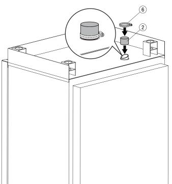
7. Insert the lower humidity vent extension into the silicon tube and secure with hose clamp
