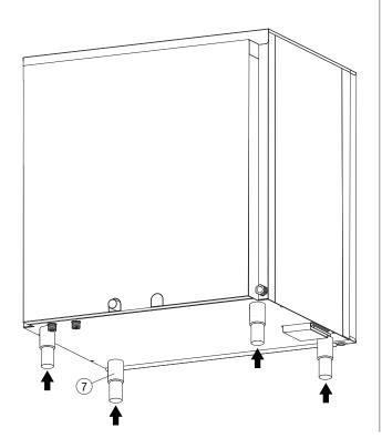
4. Using a spirit level, ensure that the Combi oven is level. Adjust the foot height to level Combi oven
