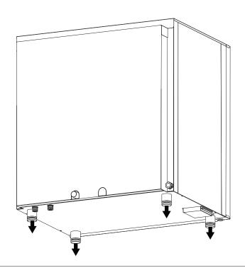
3. Install the 150mm feet to the base oven
