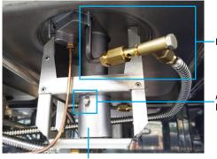
Fig.6. Air Adjustment Bush
