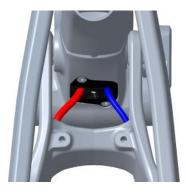
**5.** Push the cable from the rear until it appears at the head tube port. Fish it out with a pick or a bent spoke.
