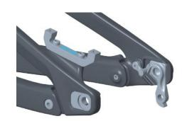
**2.** The installation of a UDH hanger requires the use of the UDH Stopper (item #65 in the Full List of Parts) to limit the rotation amount.
