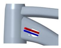
**6.** Before you re-attach the hose to the brake lever, install the foam sleeve over the hose. You will need to push the foam housing down the hose until it is fully inserted inside the frame.
