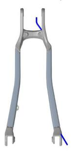
**4.** Guide the housing into the housing port above the bottom bracket. Make sure you insert the derailleur housing into the port labeled "Shift."
