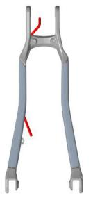
**4.** Guide the brake hose into the housing port above the bottom bracket. Make sure you insert the brake housing into the port labeled "Brake". Any brake port will do.
