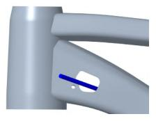
**6.** Install the foam sleeve over the housing. You will need to push the foam down the housing until the foam is fully inserted inside the frame.
