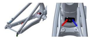
**5.** Push the brake hose from the rear until it comes out at the head tube port. Fish it out with a pick or a bent spoke.
