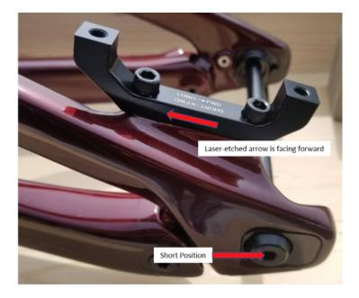
Long ----> FWD means the arrow should be pointing forward when the axle is in the long position.
