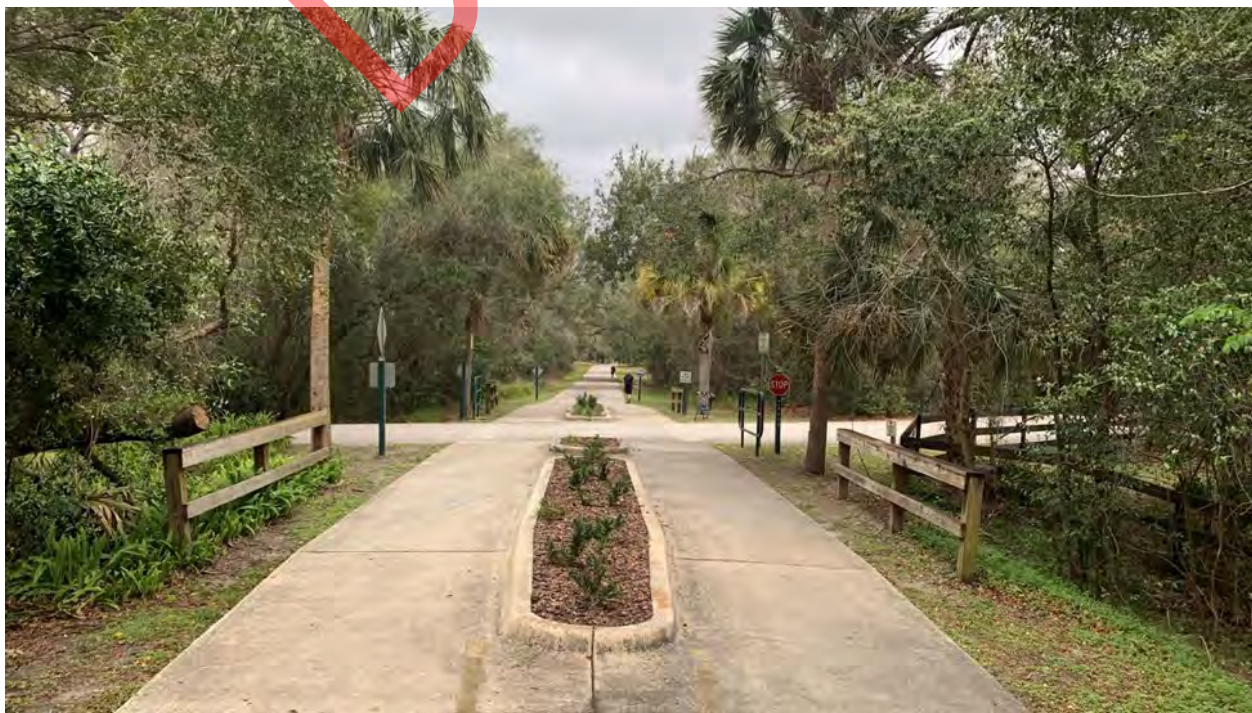
Figure 23. Use of median to restrict vehicle access
