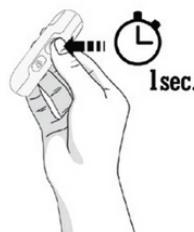
**To turn ON the device:** press the CALL button for 1 second, all the LEDs will flash rapidly.
