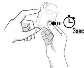
**To turn OFF the device:** press and hold the side button and SOS button together for 3 seconds until the LEDs turn off.
