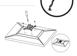
3 Fasten the Mounting Plate (included with arm) to the Crossbar with the screws provided with the arm. The Crossbar Mounting Plate should be positioned so that the arrow on the Mounting Plate is visible.
