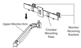
6 Align the Monitor Mounting Plates with the Monitor Receiving Brackets and slide them down until you hear a click.
