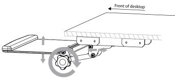
3 Rotate the knob to adjust the Keyboard Tray to find your most comfortable typing position.
