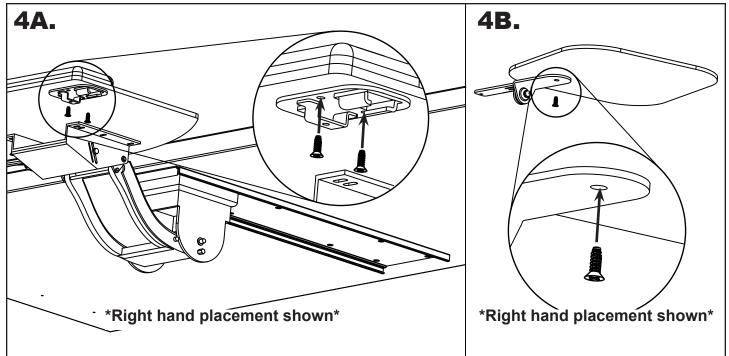
Determine if you want a right or left handed placement. Install bracketry on side that you want to install the mouse tray using (1) screw. Install bracketry onto mouse tray using (1) screw.
