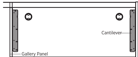
Panel system with cantilever support.
