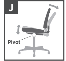
J. Synchro-tilt — Back reclines at a 2-to-1 ratio to seat angle. Allows user to recline while keeping seat cushion relatively level to floor.
