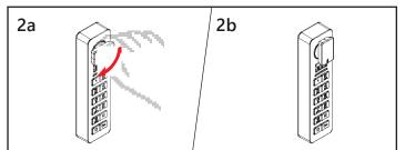
To lock: Close the door then turn the knob to the locked position.
