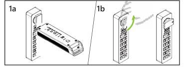
**To unlock:** Insert a valid Manager Key then turn the knob to the unlocked position. Open the door.
