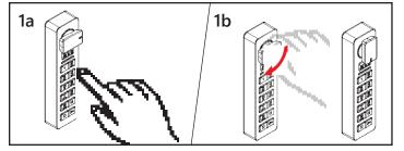
To lock: Close the door. Press C [any 4-7 digit user code] C then turn the knob to the locked position.
