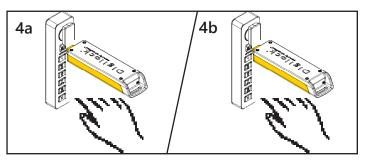
End Express Registration mode.\* Go to any programmed lock. Press: CIP then insert the Programming Key.
