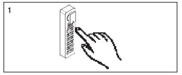
Go to a lock already programmed to operate with the Manager Keys. Press: COM 61 Om. The LED will flash.
