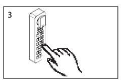
While the LED is on, Press C [new 4-7 digit user code] C C [the same 4-7 digit user code] C
