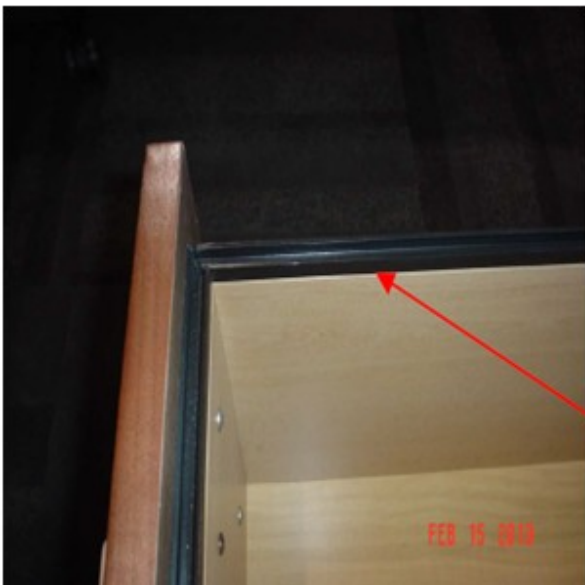
Current Hangrails— Hangrails connect to 'U' shaped mechanism within drawer side
