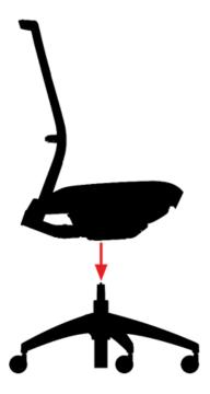
4. Apply downward force to the seat to affix the chair frame to the base assembly.
