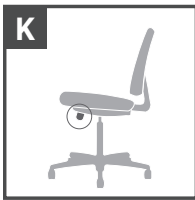
K. Tilt tension — Controls rate and ease of recline.
