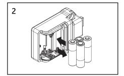
Remove the batteries from the housing. Replace with four premium alkaline AA batteries. Dispose or recycle used batteries according to local regulations.
