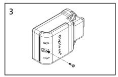
Replace the Cover Plate and secure with the screw.
