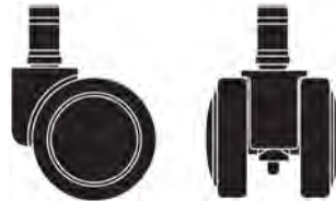
(B) Soft Wheel Wheel Diameter 2"
