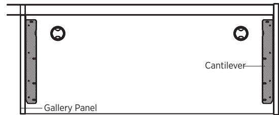
Panel system with cantilever support.
