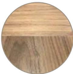
Matched veneer slices arranged with top slice rotated 90°
