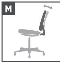
M. Posture mechanism/lock — Back angle adjusts independently of seat, and can be locked in an infinite number of positions within a fixed range.
