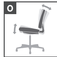
O. Asynchronous control — High performance system with three levers to modify: angle of back relative to seat, tilt (free float or infinite locking) and forward tilt.
