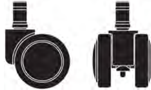
(B) Soft Wheel Wheel Diameter 2"
