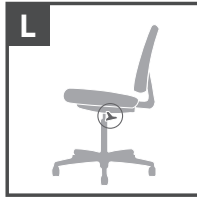
L. Tilt lock — Locks out tilt function.
