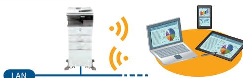
**Access Point mode\*** wirelessly connects a LAN-wired MFD to mobile PCs/devices without going through a wireless LAN router.
