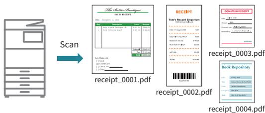
**OCR\*** OCR capability on this MFD lets you convert a scanned document into a searchable PDF file or into an editable Office Open XML (pptx, xlsx, docx) file.
