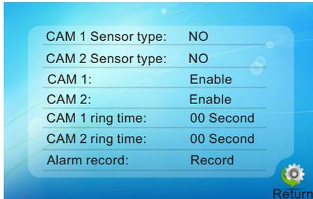
**[CAM 1 Sensor type or CAM 2 Sensor type]:** Each camera channel corresponds to an I/O status (see the following status explanations), which means that when an alarm is triggered, it will activate the corresponding channel to start alarm recording or capture a snapshot.
