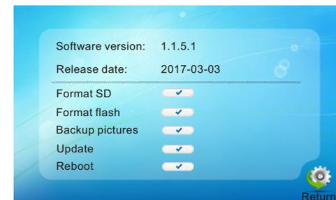
**[Format SD]:** This option is for the models with SD card. Format SD card, please format SD card firstly before using.
