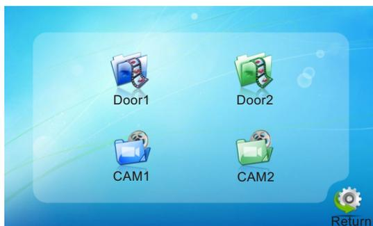
On the color menu the video color of Door1/Door2/CAM1/CAM2 attributes can be adjusted for the best image quality. Scroll the button “⚙” upwards or downwards to move the cursor to the option “Door1” or “Door2” or “CAM1” or “CAM2”, then press “⚙” to enter the corresponding menu to adjust values of brightness, contrast and chrome depending on the actual conditions.
