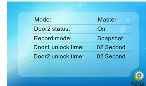
**[Mode]:** Options include "Master" and "Slave". "Master" indicates that the indoor unit connects the outdoors or cameras, "Slave" indicates that the indoor unit connects the main or sub indoor unit.
