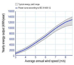
Data measured according to IEC 61400-12 standard
