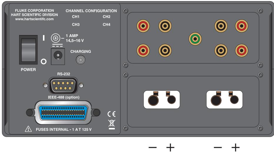
Figure 5 Thermocouple Connections
