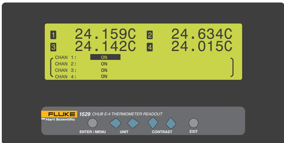
Figure 9 Enable Channel
