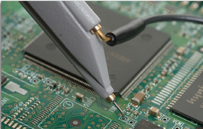
Hard-to-reach spaces can be probed with the Bent Sharp Tip and can be used with a range of ground leads like the flexible Short Right-Angle Lead shown here.
