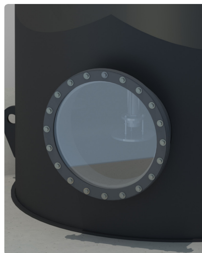
An inspection/access window is installed
