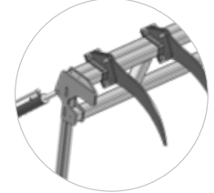
Guard frame for felling operations and to protect the tractor (option)
